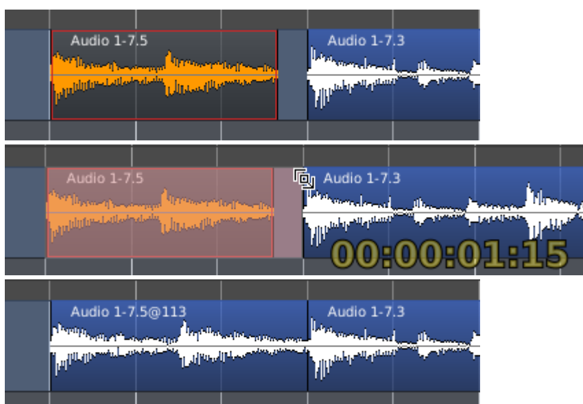
Fig. 52.3 - Using the Stretch Mode tool. Before stretching, while stretching, and after a stretch
