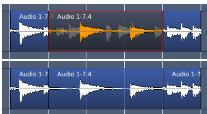
Fig. 52.5 - Region arrangement before and after 'Separate Under'
