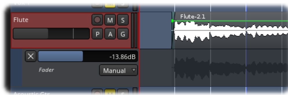
Fig. 75.3 - An example of a fader automation lane (below) with its associated track (above).
