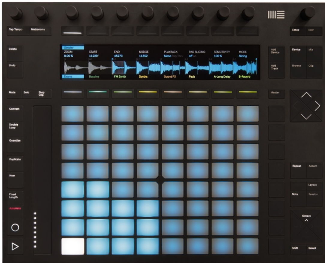
Fig. 84.1 - The Ableton Push 2 surface
