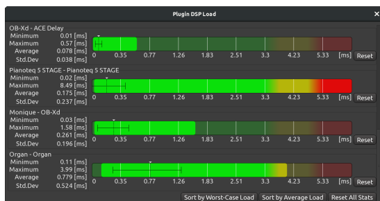
Fig. 98.1 - The Plugin DSP Load window
