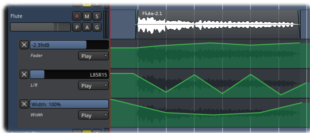
Fig. 75.5 - An example of a track with three lanes of automation (fader & pan).
