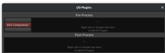
Fig. 39.4 - ACE Compressor added to the Pre-process section
