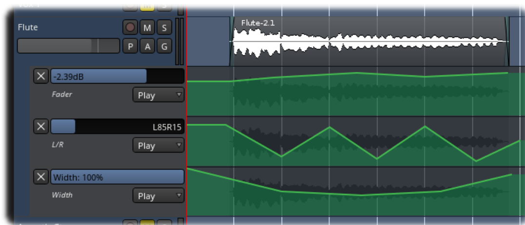
Fig. 73.5 - An example of a track with three lanes of automation (fader & pan).
