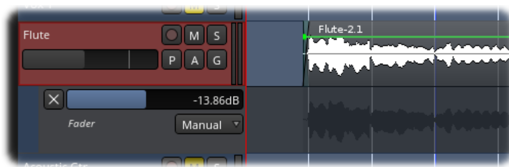
Fig. 73.3 - An example of a fader automation lane (below) with its associated track (above).
