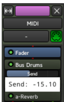
Fig. 27.4 - Connecting a bus through a send
