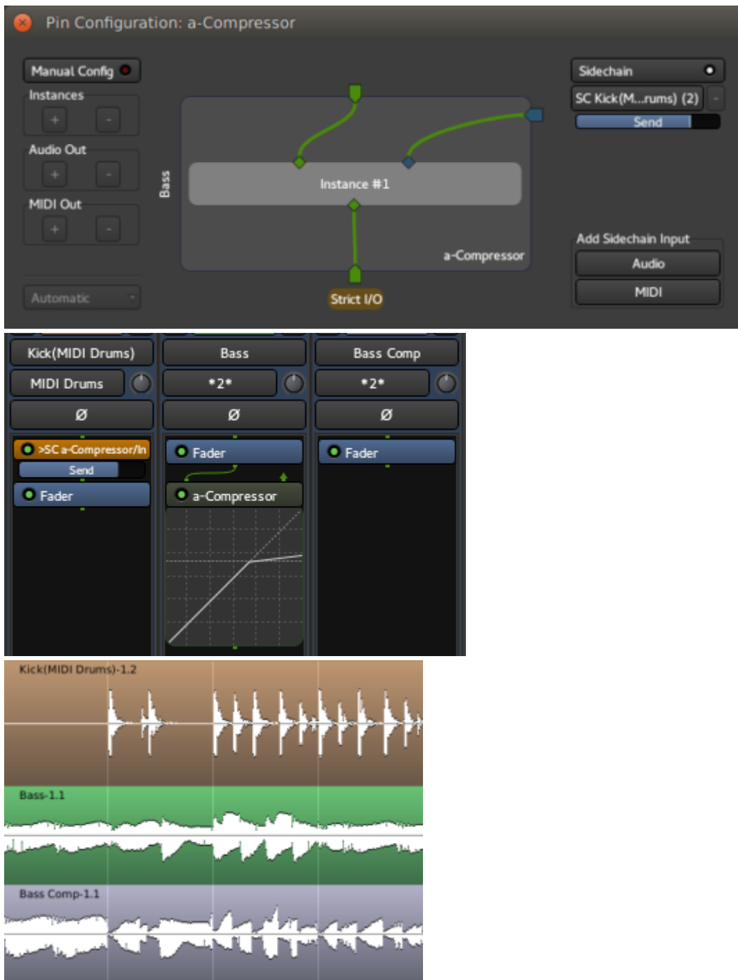
Fig. 71.19 - A sidechain compression: Pin configuration, mixer view and editor view.
