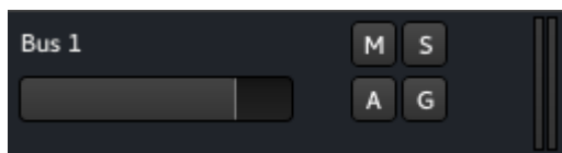
Fig. 29.5 - A bus header section
