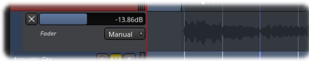
Fig. 60.1 - A typical automation lane.
