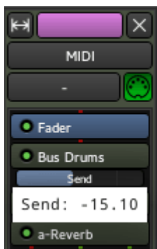
Fig. 27.4 - Connecting a bus through a send
